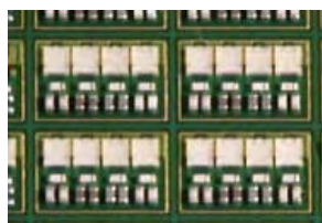
(b) After flip bonding of SAW bare chip
